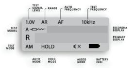
**PRIMARY DISPLAY:** The Primary Display is located in the middle of the screen and uses the largest font. It shows the dominant impedance parameter reading typically with 5 digits displayed.
