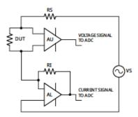
Voltage across the component is generated by the test signal source Vs. Both the amplitude and frequency of Vs can be set. The voltage is applied to the device under test (DUT) through the source
