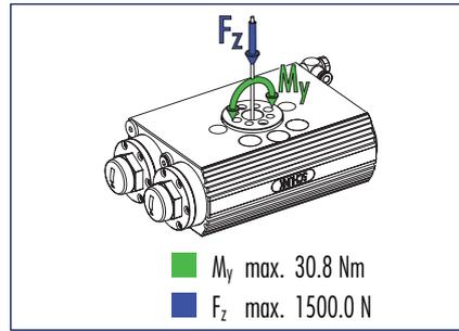
ⓘ Moments and forces may occur simultaneously. When using heavy attachments or ones with high mass moments of inertia, the speed must be restricted to ensure that the rotary movement occurs without any hitting or bouncing.
