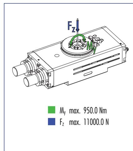
ⓘ Moments and forces may occur simultaneously. When using heavy attachments or ones with high mass moments of inertia, the speed must be restricted to ensure that the rotary movement occurs without any hitting or bouncing.
