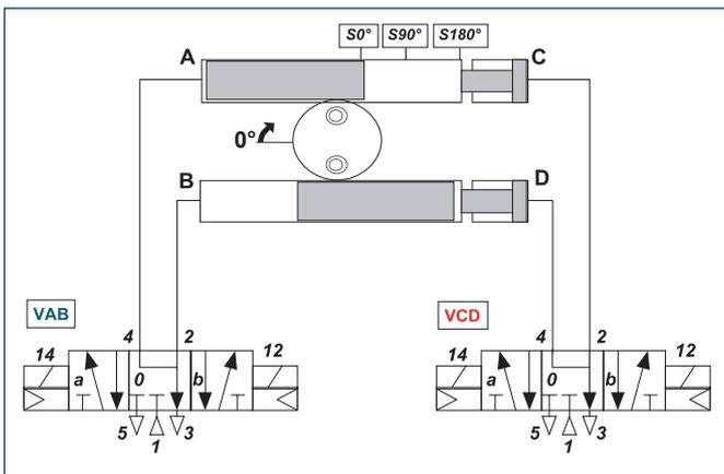
VM units with vertical swivel axis are generally actuated by two 5/3 directional control valves with bled center position. To prevent damage, it is essential that you pay attention to the actuation sequence in the Operating Manual.
