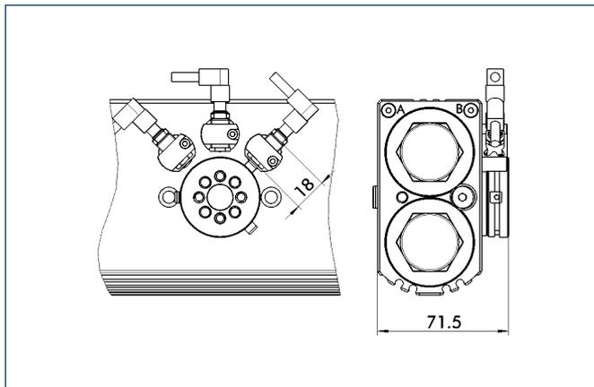
The size-specific mounting kit is required for installing the inductive proximity switches. Up to three proximity switches (2x end position, 1x center position) can be attached using the mounting kit. A mounting kit for IN 80 inductive proximity switches consists of:
