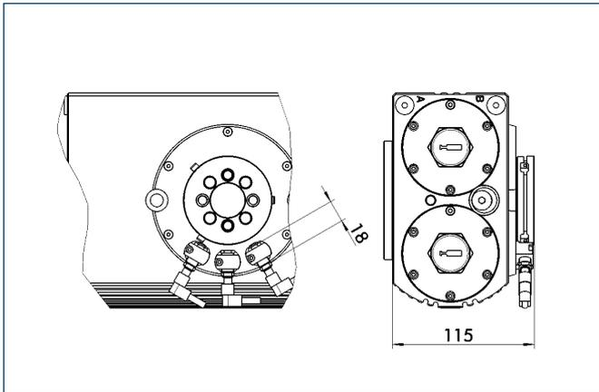
The size-specific mounting kit is required for installing the inductive proximity switches. Up to three proximity switches (2x end position, 1x center position) can be attached using the mounting kit. A mounting kit for IN 80 inductive proximity switches consists of:
