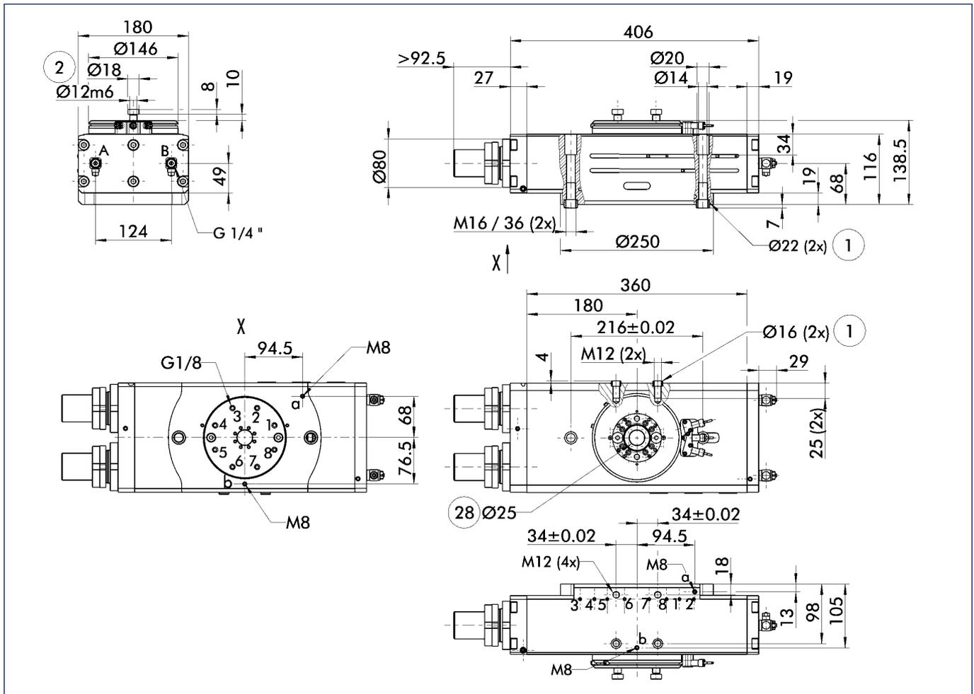
The main view shows the SRU in the most basic version, that is with an angle of traverse of  $180^\circ/90^\circ$ , small end position adjustability of  $3^\circ$ , without center position and without fluid feed-through. Modifications to the drawings as a result of various options can be seen in the relevant additional views.
