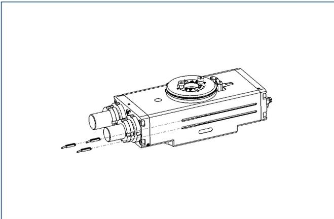
End position monitoring: Electronic magnetic switches, for mounting in C-slot
