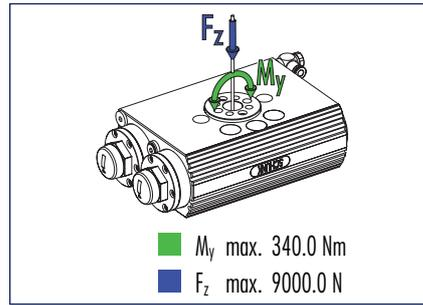
① Moments and forces may occur simultaneously. When using heavy attachments or ones with high mass moments of inertia, the speed must be restricted to ensure that the rotary movement occurs without any hitting or bouncing.
