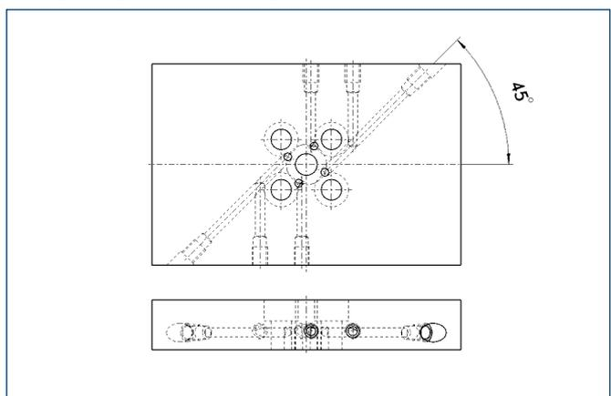
Suggested here is an arrangement of the adapter plate which enables all fluid feed-throughs to be reached as easily as possible.
