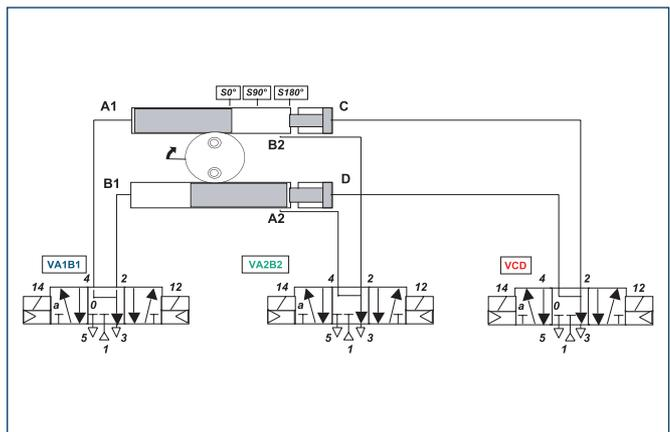
VM units with horizontal or non-vertical swivel axis must generally be actuated by three 5/3 directional control valves with bled center position. To prevent damage, it is essential that you pay attention to the actuation sequence in the Operating Manual.
