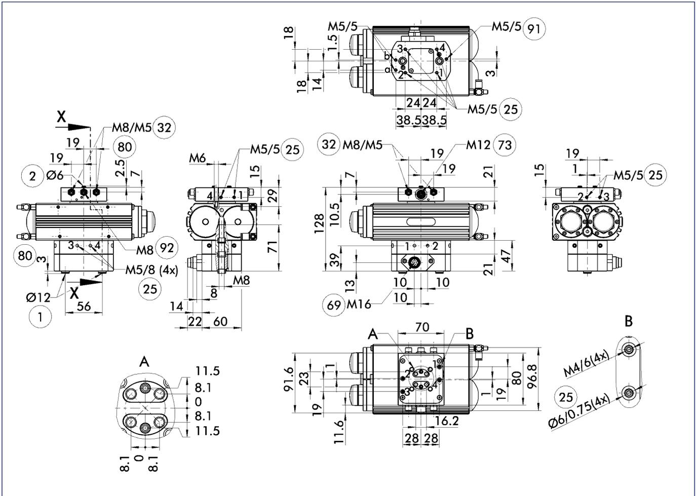
The main view shows the SRU in the most basic version, that is with an angle of traverse of 180°/90°, small end position adjustability of 3°, without center position and without fluid feed-through. Modifications to the drawings as a result of various options can be seen in the relevant additional views.
