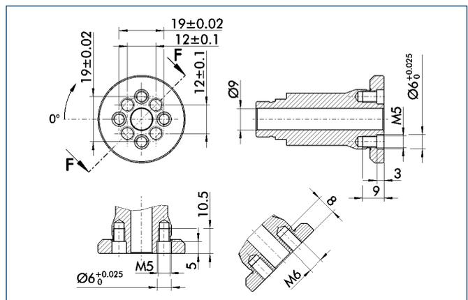
Pinion screw connection diagram for mounting the swiveling attachment. The „4x large thread for 4x screw and 2x flat fit for guide sleeve“ screw connection diagram is preferable to the „4x small thread for 2x screw and 2x dowel screw“ (in deep fit) screw connection diagram.
