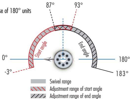
Small end position adjustability ( $\pm 3^\circ$ ) for fine adjustment
