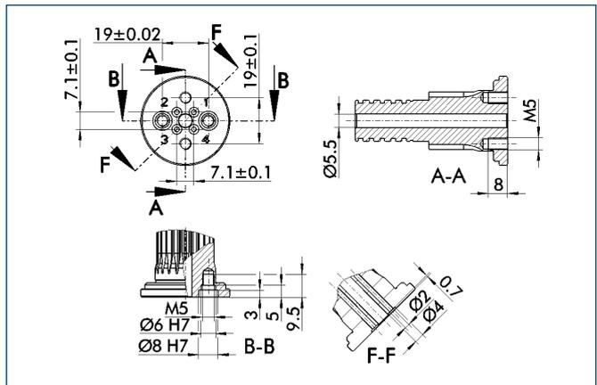
Pinion screw connection diagram for the „Fluid feed-through“ option. The preferred drilling pattern is 2 x screws and 2 x screws with guide sleeve (in ø 8 H7).
